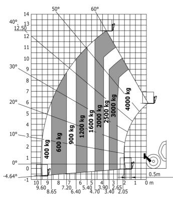
Machine on lowered stabilisers with forks Metric
